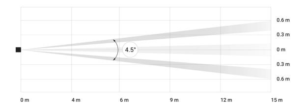
Horizontal viewing angle of the detector
