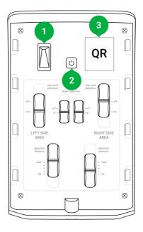
**1.** Tamper button. Triggers when an attempt is made to detach the detector from the surface or remove it from its mounting
