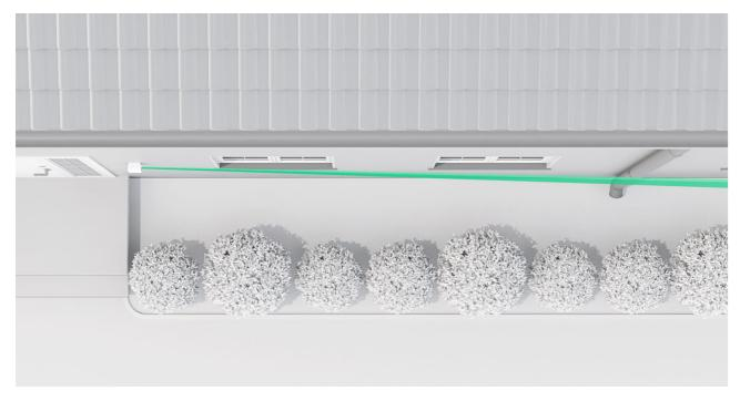
If appropriate, turn on **Near area detection** (**Near area detection** scrollbar) for the desired side. The mode allows the detector sensors to detect motion when an attempt is made to break in at the very body of the device, reducing the blind spot.
